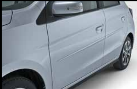
▲ Side protection moulding Painted in body colour. For part numbers see quick reference list.
